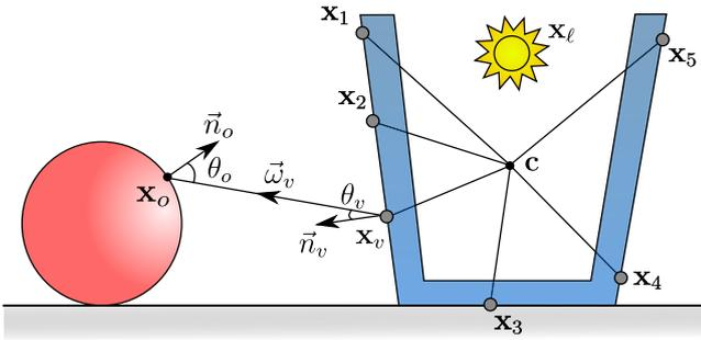
**Fig. 5** Transport of emergent light from a translucent object (blue) to a diffuse object (red). We distribute VPLs (gray dots) on the outer surface of the translucent object, and use them to indirectly illuminate the remaining scene.
