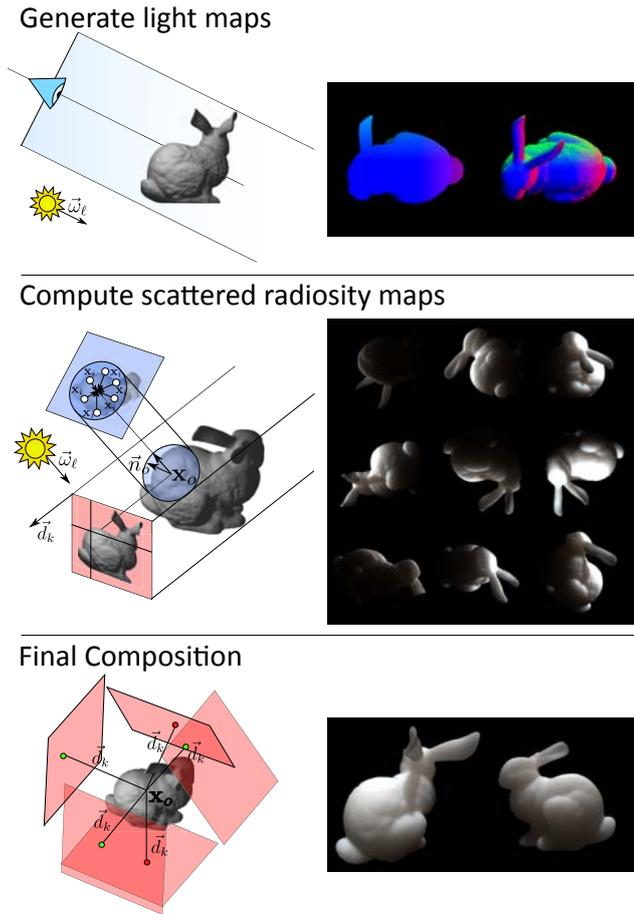
**Fig. 3** Our three-step multipass technique for interactive rendering of directional subsurface scattering in deformable translucent objects. The scattered radiosity maps enable view-independence and transport of emergent light.
