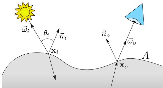
**Fig. 2** BSSRDF configuration on an object surface  $A$ . The diagram illustrates the notation we use: bold font as in  $\mathbf{x}_o$  denotes a point, while arrow overline as in  $\vec{\omega}_i$  denotes a normalized direction vector.
