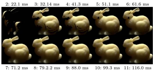
**Fig. 13** Converged renderings of a potato bunny ( $N = 30$ ) and timings for increasing number of scattered radiosity maps  $K$ . We list  $K$  followed by rendering time in milliseconds (ms) for each result. The first 7 maps cover most of the surface, while the following 4 cover small details (the small area just to the left of the bunny’s hind leg, for example).
