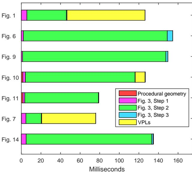
**Fig. 12** Timing breakdowns for some of our renderings. Initialization times were negligible and were thus included with step 1 of Fig. 3. The evaluation of the BSSRDF and the VPLs (when present) dominate the rendering times.
