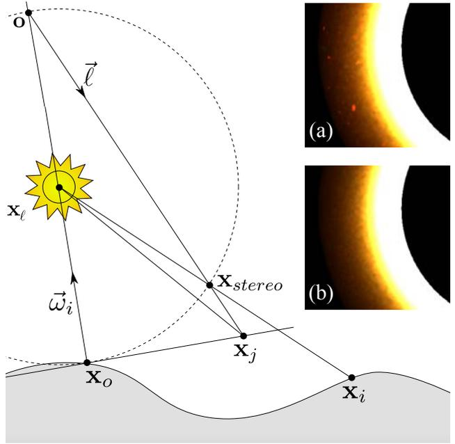
**Fig. 4** Effect of stereographic correction when a translucent object surrounds a point light. With planar sampling (a), we look up into the light’s cube map G-buffer using  $\mathbf{x}_j - \mathbf{x}_\ell$ . With stereographic correction (b), we use  $\mathbf{x}_{\text{stereo}} - \mathbf{x}_\ell$  instead. The insets (a and b) show how the correction improves the final result (torus, potato material).
