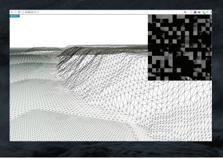
Figure 2. Caching and Level of Detail in rendering. The upper right corner shows the height map tiles that are streamed into the graphics card memory.
