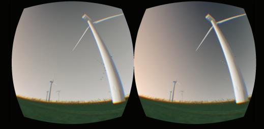
Figure 3. The image shows stereoscopic rendering for each eye. When viewed through the lenses of a VR helmet, sizes, distances and colors will appear as if they were real.
