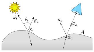
Fig. 2 BSSRDF configuration on an object surface A. The diagram illustrates the notation we use: bold font as in  $x_o$  denotes a point, while arrow overline as in  $\vec{\omega}_i$  denotes a normalized direction vector.
