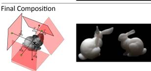
Fig. 3 Our three-step multipass technique for interactive rendering of directional subsurface scattering in deformable translucent objects. The scattered radiosity maps enable view-independence and transport of emergent light.
